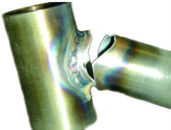
Figure 40. The fracture in this steel alloy tube is about 1/8" (3 mm) to the right of the weld, and is an acceptable fracture as a result of excessive force.
