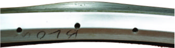
Figure 54. Cracked rim as a result of excessive spoke tension. Although not impossible to occur at the front wheel, this event is most common on the right (drive) side spokes of the rear wheel, because of the rear hub's rotational force transmitting from the spokes to the rim.
