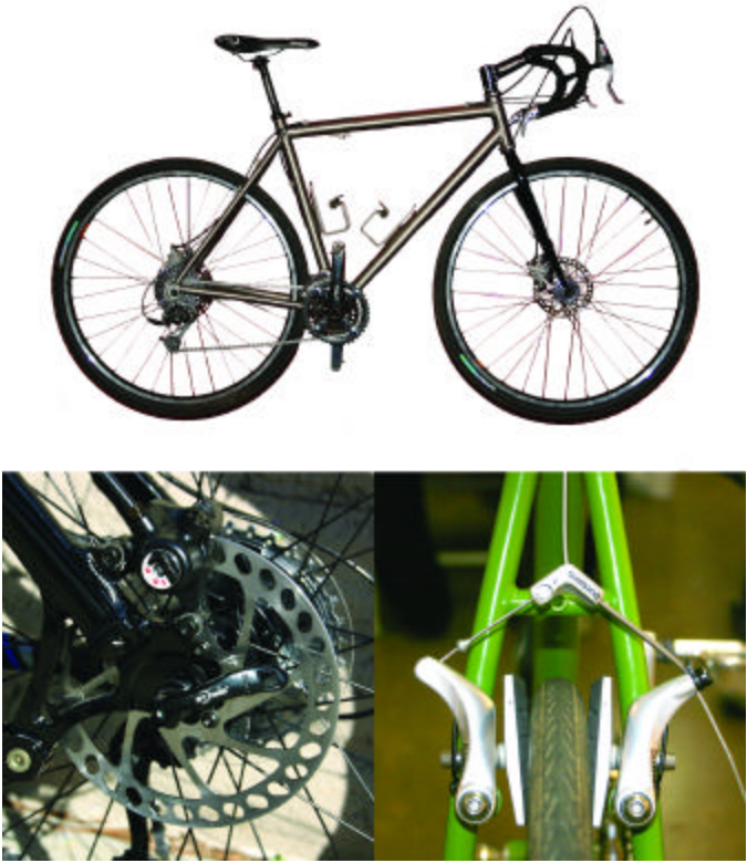
Figure 28. The Cyclo-cross usually is equipped with slightly-knobby and narrow 700mm wheels, multiple-speed gears, and drop handlebars. Cantilever brakes (lower right) are the most common, but some have disc brakes (lower left). Although similar in appearance to a Road/Race bicycle, the Cyclo-cross differs in that the fork is usually straight, rather than curved, and the frame is a size or two smaller to ease dismounting. The fork, brakes, and stays are usually designed for optimum mud clearance. The titanium model above was designed with 73-degree seat and head tubes, which are common angles for this bicycle type.
