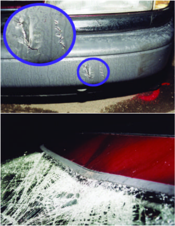
Figure 74. The upper image depicts a bicycle pedal imprint on the front bumper cover of a minivan involved in a right-angle collision, while the lower image depicts an head/shoulder imprint at the top of the windshield and leading edge of the roof. From the driver's view, the bicycle was traveling from left to right. The location of the damage in the lower image is further inboard from the driver's side than the location of the damage in the upper photo, indicating that the bicycle was moving at the time of impact.
